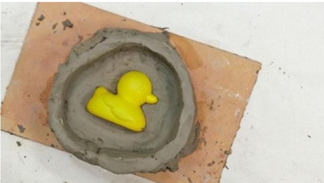
This video shows the making of a press mould of a 3D object. The most important part of this process is finding the casting lines. If your object has undercuts the plaster mould will grip to the original. We have chosen a very simple example to demonstrate, a plastic duck. If your object is more complicated or not plastic, you will need to use a liquid soap release agent to help the original come away from the mould.
